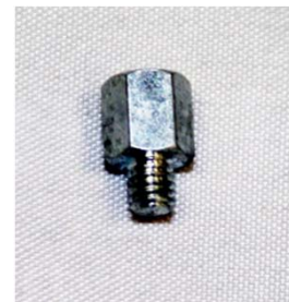
Distance holder for the DC-DC board
